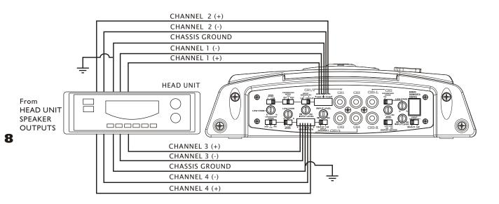
Note: Use the 4CH mode when using high level (speaker) inputs and the 5CH mode use with for low level (RCA) inputs.
